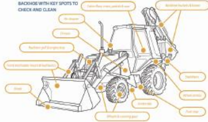
BACKHOE WITH KEY SPOTS TO CHECK AND CLEAN
